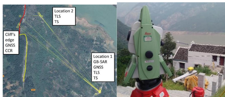
Figure 4 Left: TS network and sensors used at each location (Background source: Google Maps©), right: example of setup at location 1 with TS, GB-SAR and GNSS Receiver
